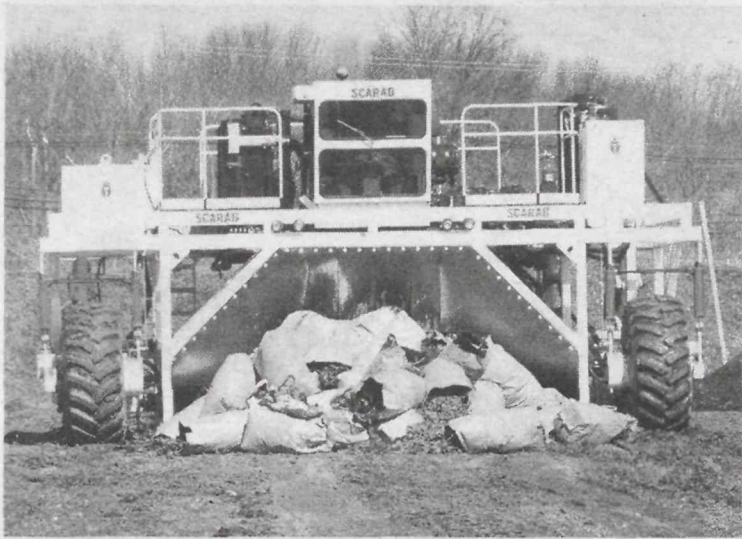
Middlesex County Improvement Authority's windrow turner turns and fluffs curbside by way of a rotating drum with fins.
