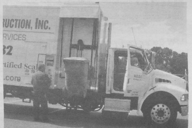
Mobile shredding vehicle with recycling material traveling to top of the truck to be shredded.
